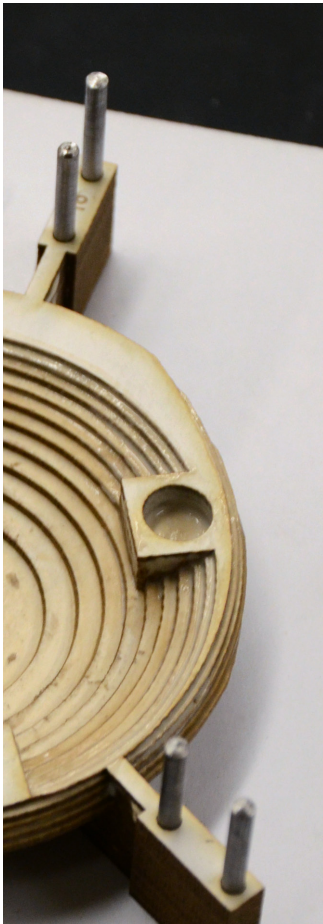
Embedding a magnet during the stacking of the layers.
