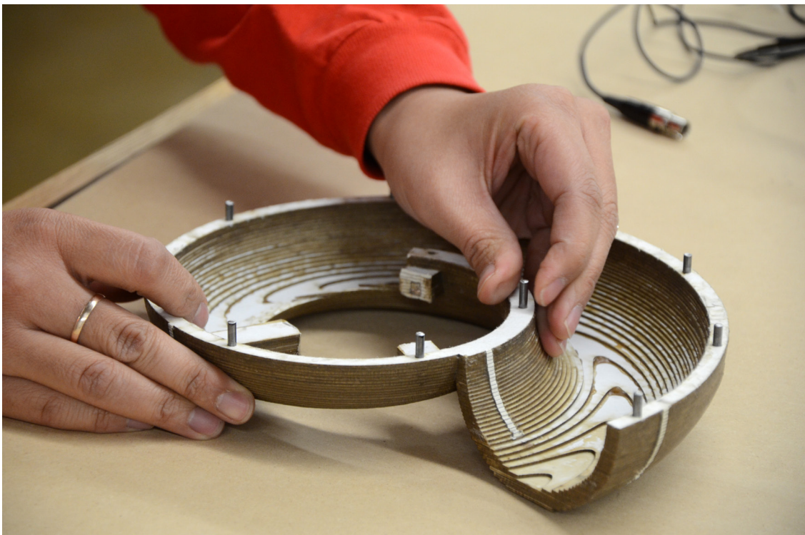
Installing guide pins for the body.
